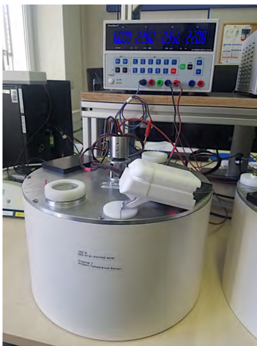
Figure 5.1: SHC with a candidate radiosonde measuring during the UAI campaign. The power supply for the fan motor is on the rack in the background.
