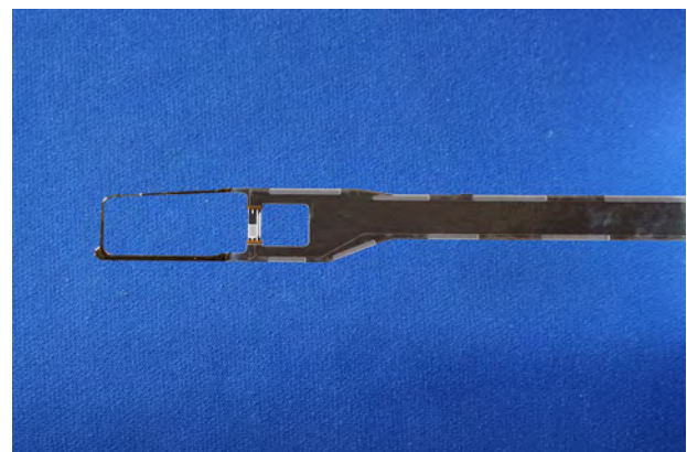
(b) Sensor boom of RS41
