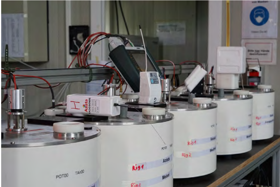
Figure 4.12: Set of five 100 %RH SHCs with the manufacturer-independent ground check running in four of them.
