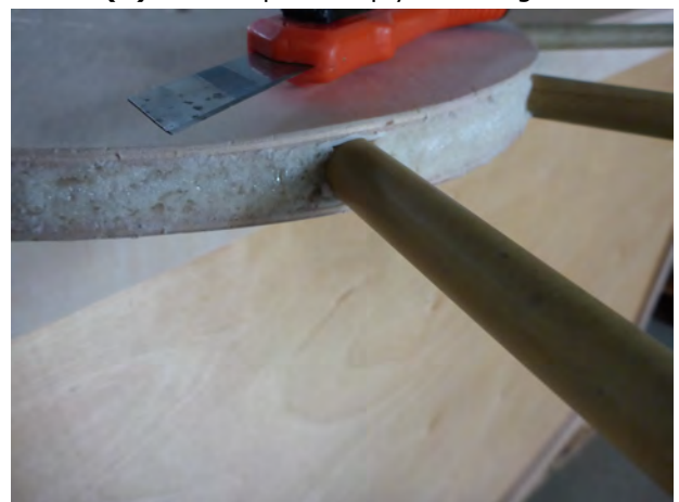
(f) Remove excess material with the cutter
