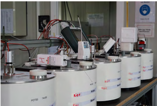
(e) Standard humidity chambers (SHC) for 100% ground checks
