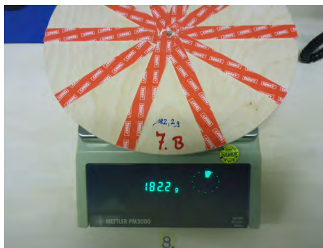
Figure N.3: Weighing a plywood plate
