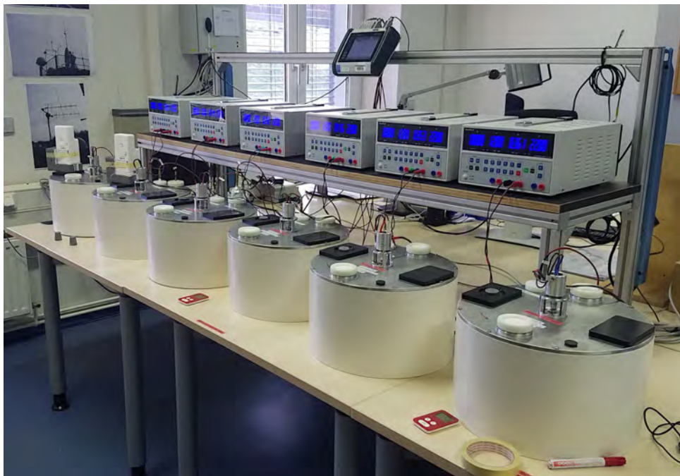
Figure 5.2: Laboratory setup for UAI relative humidity calibration checks. The data acquisition system for the reference sensors is mounted on the rack above the power supplies. The SHCs are lined up with increasing humidity from right to left.
