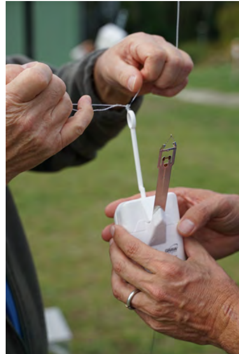
(b) Attaching a radiosonde
