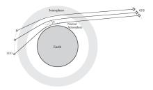
Phase shift  $\rightarrow$  bending angle  $\rightarrow$  refractivity  $\rightarrow$  (dry) temperature
