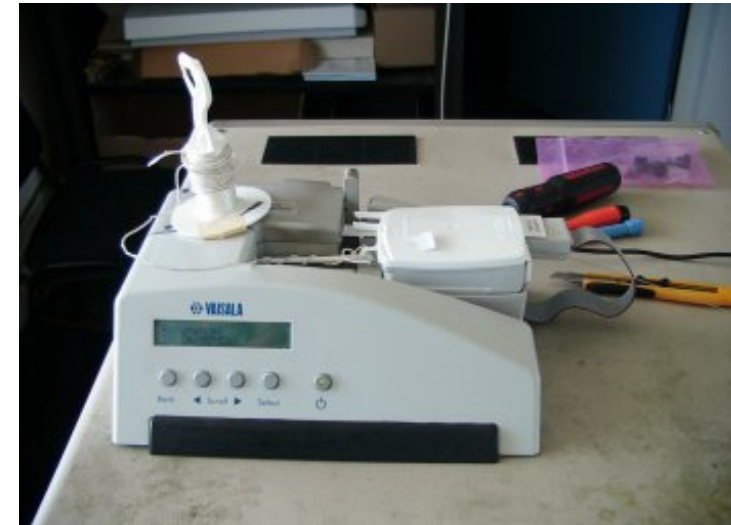
Use of Standard Humidity Chamber at 100% (2006-2014)
