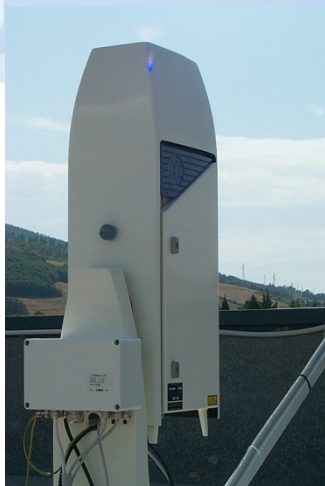
CT25K 905 nm ceilometer Operational since August 2004
