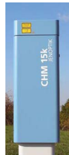
CHM15K 1064 nm ceilometer Operational since July 2009
