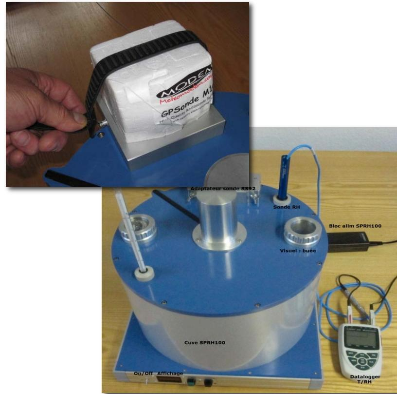
RH measurement in saturated environment using SPRH100
