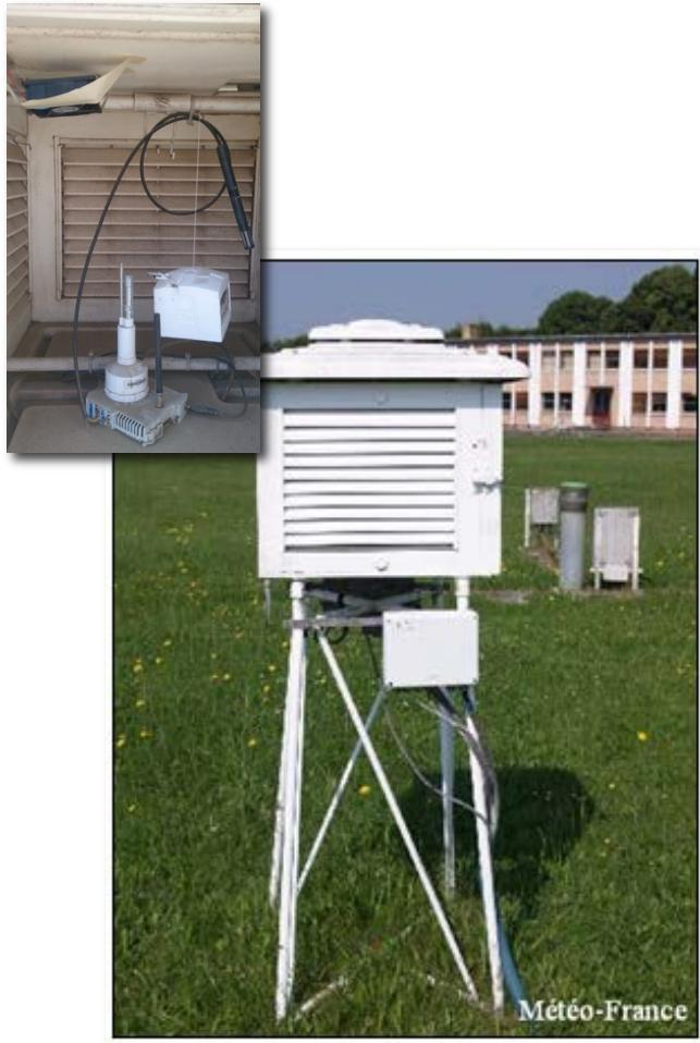
Comparison with calibrated temperature and RH sensors in ventilated hut – ambient conditions
