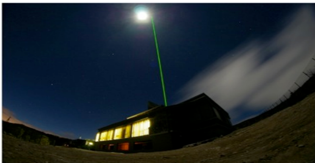
Water vapor Raman lidar beam 1.2m diameter telescope, Dual Q-R laser Vaisala and Modem ground stations
