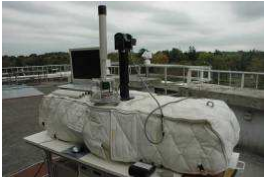
Dobson ozone spectrophotometer
