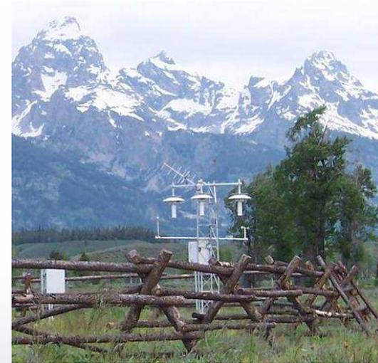
Triplicate sensors allow detection of equipment problems and ensure data quality and continuity
