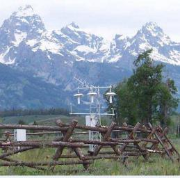
Triplicate sensors allow detection of equipment problems and ensure data quality and continuity
