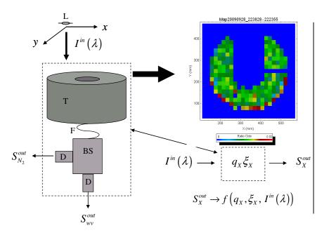
•The water vapor mixing ratio calibrationRD factor  $C_R$  depends on the optical TY efficiency ( $\kappa$ ), the differential scattering cross sections  $(d\sigma/d\Omega)$  and the band pass filter shape ( $\epsilon$ )
