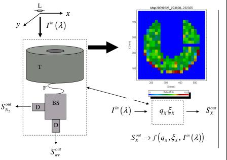
Ignoring cross section errors, one can obtain 3% relative uncertainty in *CR* with careful optical filter characterization.
