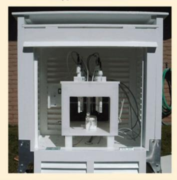
The THref uses 6 research-quality T/RH probes in a fan-ventilated chamber within an instrument shelter to provide an accurate time series of surface conditions. A photosensor signal marks the presence of a radiosonde in the THref data file, for later correlation and comparison of the radiosonde and THref measurements.
