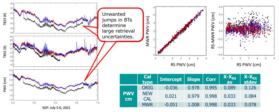
Black: Original Blue: New cal Red: 2-channel MWR Yellow: RS The **re-calibration** reduces scatter in water vapor retrievals by eliminating unwanted jumps in the BT and it **makes the new measurements consistent with the old 2-channel MWR measurements ensuring good continuity of the dataset despite the change of instrument.** The new PWV (blue) has improved bias and standard deviation compared to the original PWV (black)
