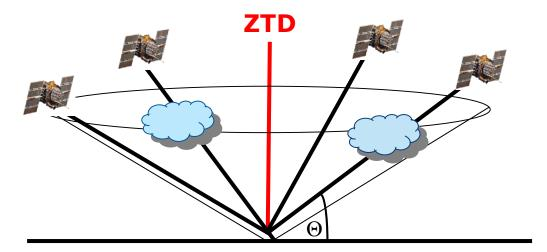
Isotropic water vapor distribution & known mapping function ( $\sim 1/\sin \Theta$ )
