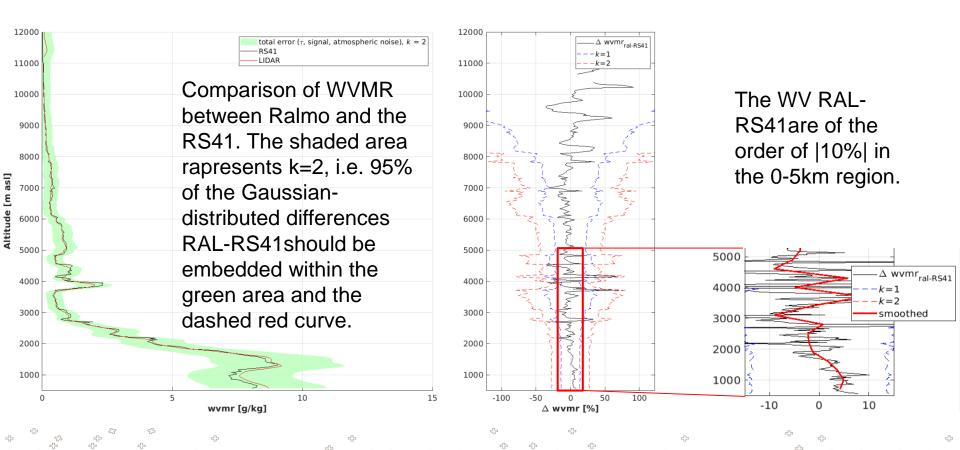
From 7.7.2021 to 31.10.2021, profiles of WVMR have been compared to the profiles obtained by the operational sonde Vaisala RS41 at Payerne and assessed separately for daytime and nighttime (76 and 72, respectively) based on the bias and standard deviation
