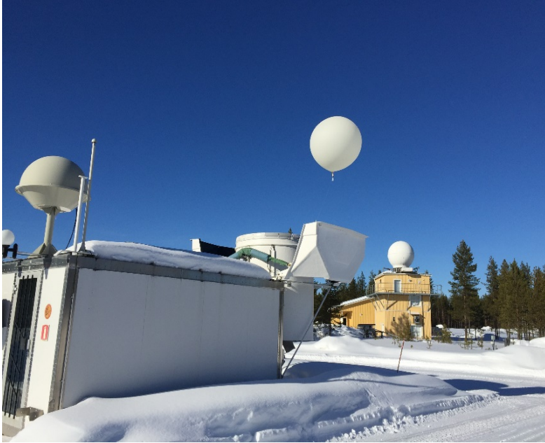
Vaisala AS41 autsonde system operational at the Finnish Meteorological Institute GRUAN site in Sodankylä
