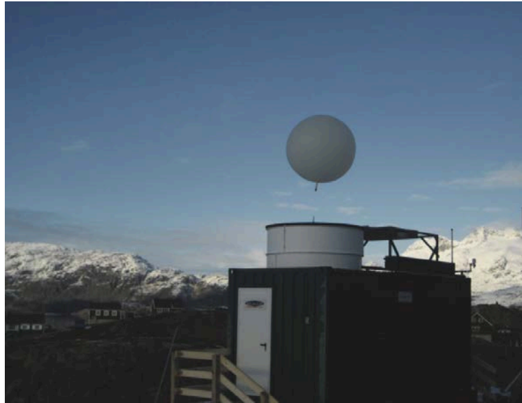
Modem Robotsonde launching a balloon at Station Tasiilaq (WMO index = 04360, photo from https://www.dmi.dk/fileadmin/user_upload/Rapporter/TR/2015/DMI-TR-15-12.pdf )
