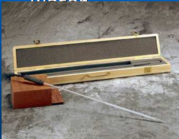
Standard Platinum Resistance Thermometer (SPRT): interpolates between fixed points
