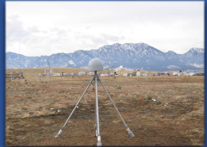
Global Positioning System instrument measuring total column water vapour at Boulder, Colorado, USA
