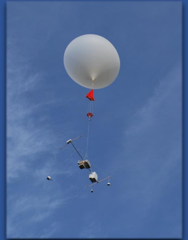
Balloon lifting several radiosondes as part of a regular intercomparison at Lindenberg, Germany.
