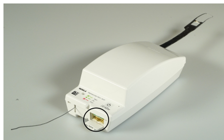
(a) Vaisala RS41 radiosonde with opened additional sensor interface port right hand from the antenna (marked with a black circle).
