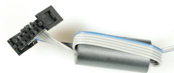
(b) Assembled wire housing and wire with one turn on a ferrite tube.
