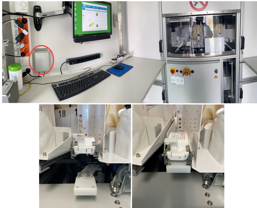
Figure 3.4: View into the operator room of AS15. The robot room is behind the window (top right). The ground check device RI41-AS1 is marked with a red circle (top left). Bottom: view into the robot room, with the NFC module arm approaching the RS41 for wireless communication (from left to right).
