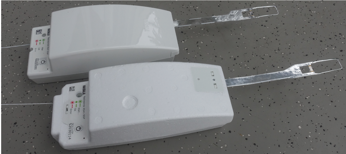
Figure 2.1: RS41-SGP radiosonde. Model with hard-plastic cover (back), and Soft & Light version with EPS foam material housing (since October 2017) (front).
