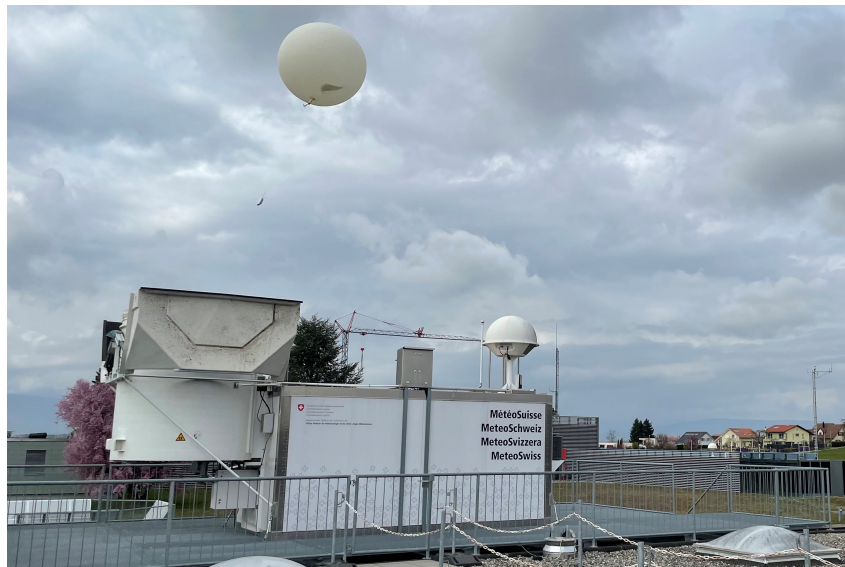
Figure 2.10: Vaisala Autosonde ® AS15 sounding station during launch of a RS41, installed at the GRUAN site of Payerne (PAY), Switzerland.
