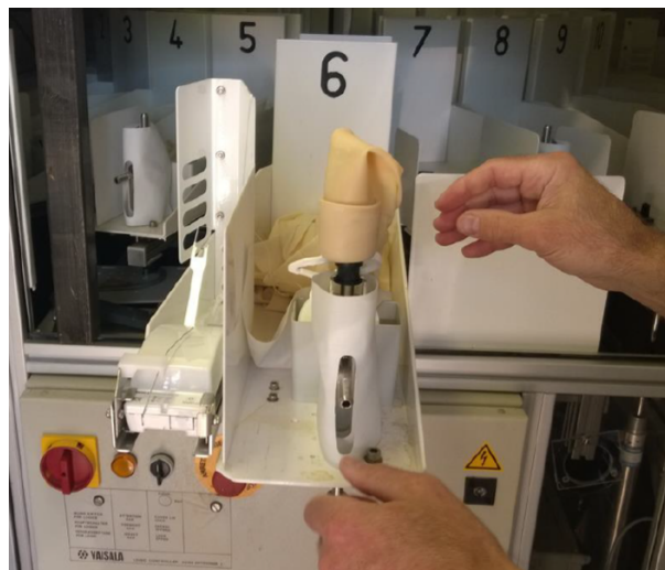
Figure 3.3: Finalisation of the balloon and payload assembly in tray 6 (out of 24) of the rotating table. A “pull-out” mechanism provides easy access to individual trays from the control room in the AS15 sounding station. Each payload is comprised of a balloon, parachute, a valve, an unwinder, and a RS41 radiosonde (photo taken from Vaisala, 2018a ).
