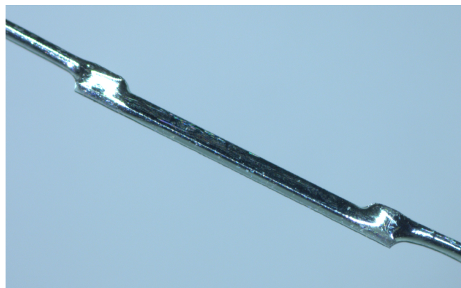
Figure 2.3: Macro photo of the Pt1000 platinum resistance temperature sensor of the RS41 radiosonde. The length of the sensor element is about 5 mm.
