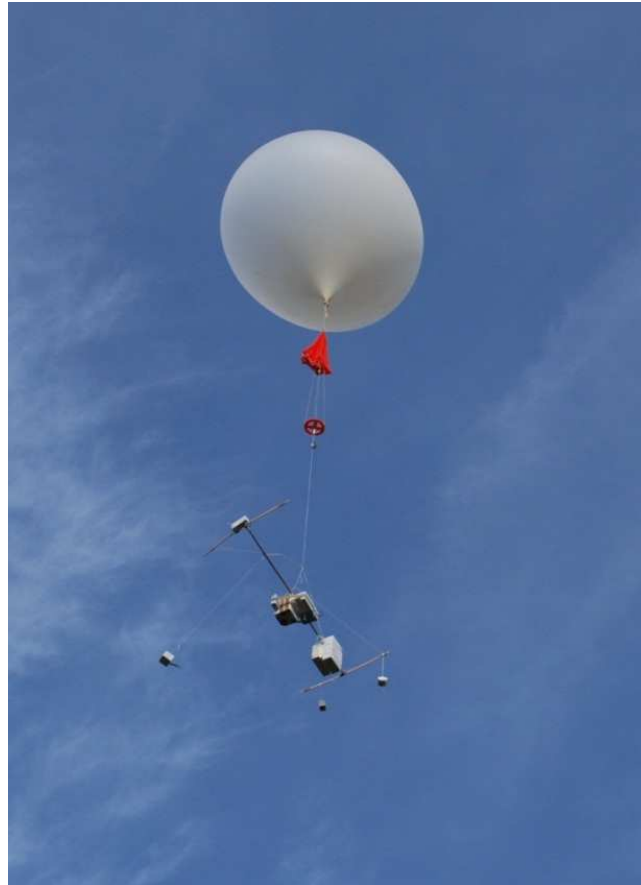
Figure 1: Example of multiple-payload rigging arrangement at Lindenberg, Germany during the Lindenberg Upper-Air Method Intercomparison (LUAMI) during 3–24 November 2008. Operational radiosondes and scientific instruments are connected by booms and additional strings, and the whole payload is attached to a single weather balloon by the main string with a red parachute inline.
