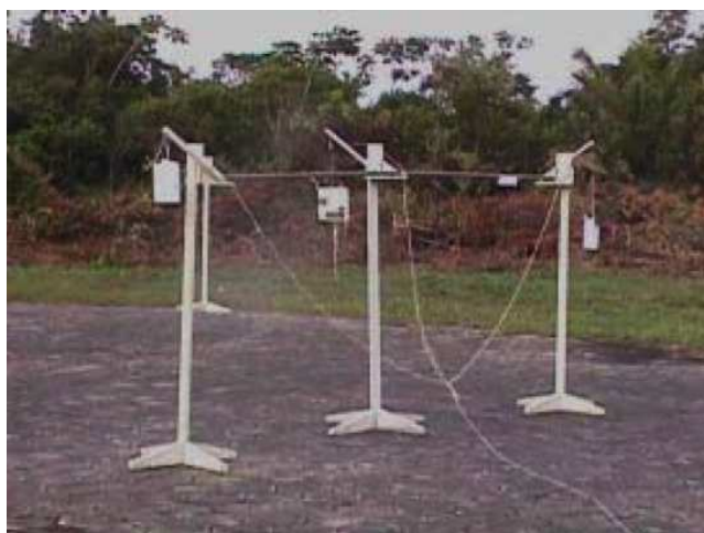
Figure 12: Photograph showing a boom with three radiosondes hanging, being prepared for balloon launch during the 2001 WMO radiosonde comparison campaign at Alcântara, Brazil.
