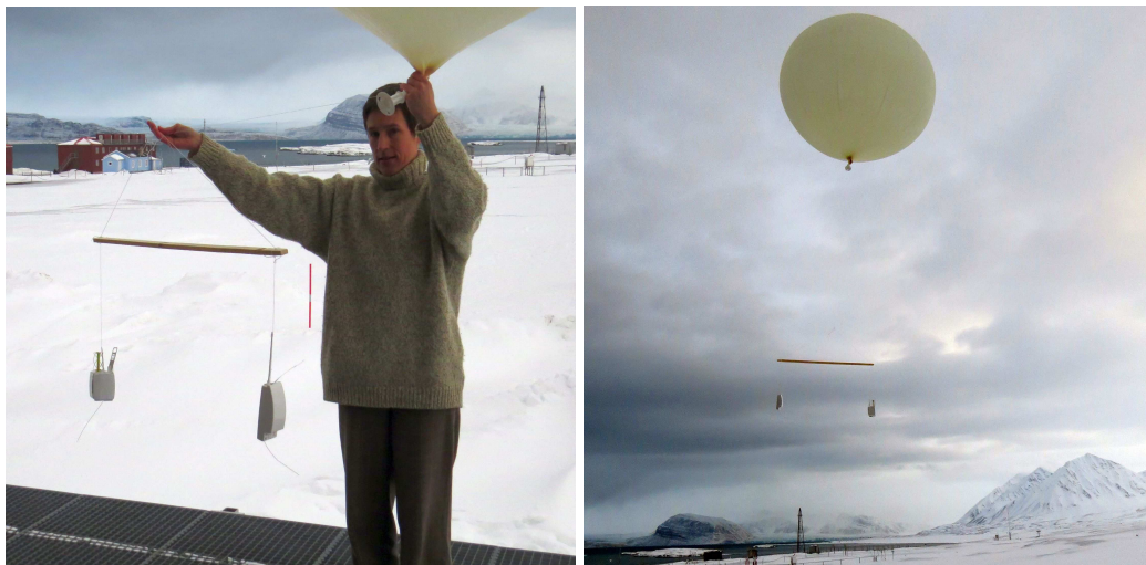
Figure 30: Photographs of a RS92-RS41 dual sounding at Ny Ålesund. The radiosonde dual soundings were performed in the framework of GRUAN, to provide simultaneous observations by the two radiosonde types, that allows for the detailed comparison and the identification of deviations.
