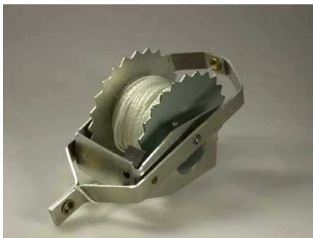
Figure 2: An example string unwinder (GRAWs model UW1 series). The string is 0.8 mm in diameter, with either 30 m (UW1-30) or 50 m (UW1-50) length. The maximum mass of the payload that can be held is 5 kg. Once launched, the unwinding speed is 0.1 \text{ m} \cdot \text{s}^{-1} for a 210 g payload and 0.3 \text{ m} \cdot \text{s}^{-1} for a 2.5 kg payload.
