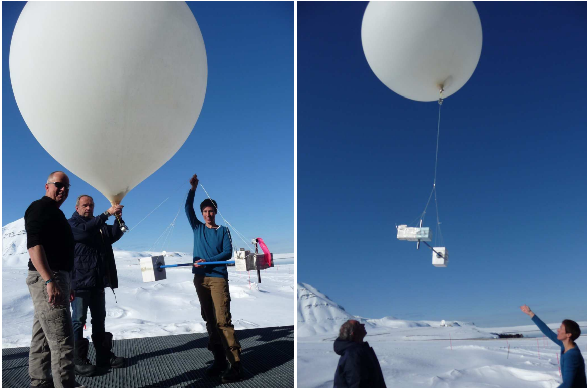
Figure 16: Photographs showing a sounding of an iMet radiosonde with CFH (Cryogenic Frostpoint Hygrometer), and a RS92 radiosonde with ECC ozonesonde fixed on a 1 m-long plastic rod, at Ny Ålesund (78.92°N, 11.92°E), Svalbard/Norway. The set-up was used in the period September 2013 to January 2017.
