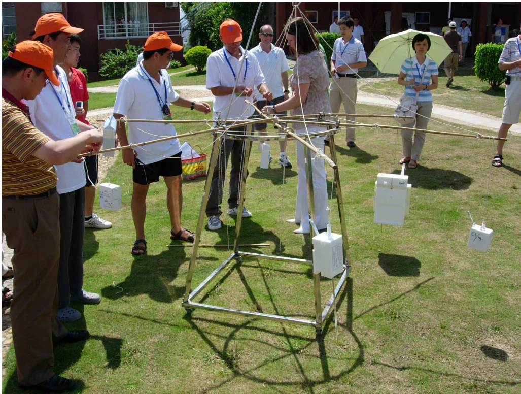
Figure 8: Preparation of a multiple-payload assembly using three bamboo booms during the 2010 WMO radiosonde intercomparison campaign at Yangjiang (21.83°N, 111.97°E), China. The \sim 3 m-long bamboo booms were temporarily situated on top of the aluminum-frame holder during preparation. A string of \sim 0.7 m length was used to hang each radiosonde from a boom (note that during the preparation period, shown in this photograph, each string was wound around the boom so that the instruments did not touch the ground).
