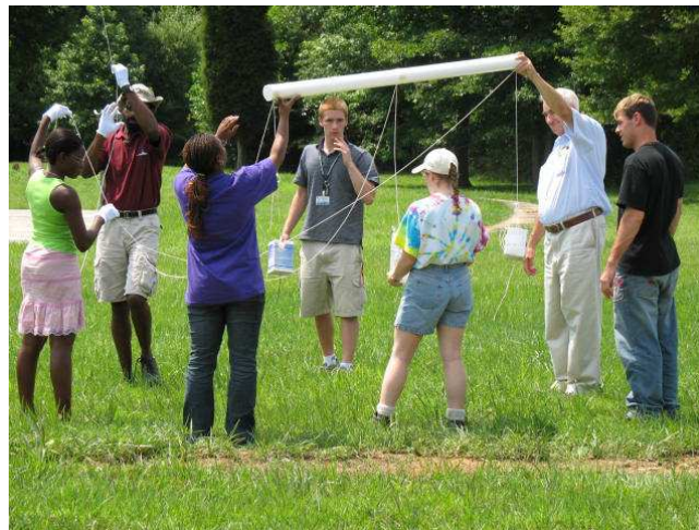
Figure 7: An example of multiple instruments hanging from a 2 meter-long boom of solid cylindrical Styrofoam. Taken at the Howard University-Beltsville site (39.05°N, 76.88°W), Washington, D.C., USA. The same boom is also used by the National Weather Service Sterling Field Support Center (SFSC) for multi-payload operations.
